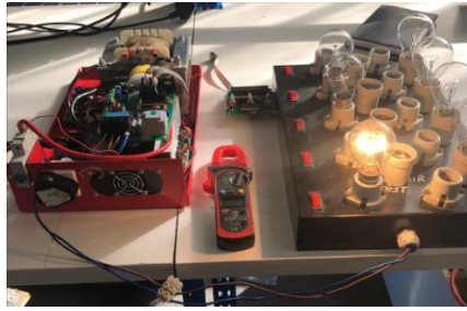
Figure 4: Load box connected to inverter
